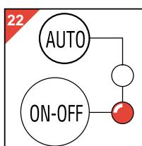
When the appliance is switched on automatically, the corresponding red pilot light will come on and the yellow light will go out (fig. 22).
