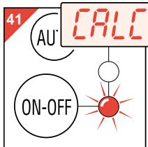
If pilot light **ON/OFF** starts blinking and the word **CALC** alternates with the actual time reading (fig. 41), your appliance needs descaling.
