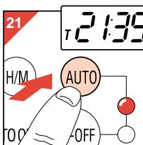
Press button **AUTO** if you want the coffee maker to switch on automatically at the set time (within 24 hrs) (fig. 21). The corresponding yellow pilot light will come on.
