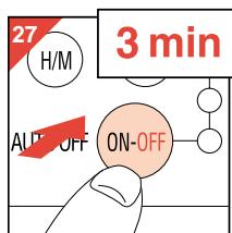
If you have made one jug of coffee and wish to make some more straight away, please switch the coffee maker off (fig. 27) and allow about three minutes for it to cool down. Then you can refill the water tank.
