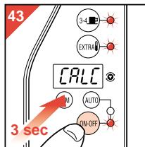
Press and hold the on/off switch for three seconds when switching on. The three red pilot lights will start blinking (fig. 43).
