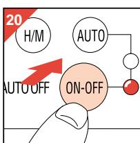
Press button **ON/OFF** if you want the coffee maker to start brewing rightaway. (Thus without using the timer) (fig. 20). The corresponding red pilot light will come on .
