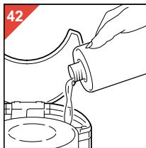
Fill the water tank with **ordinary vinegar** and do not place a filter with ground coffee (fig. 42).
